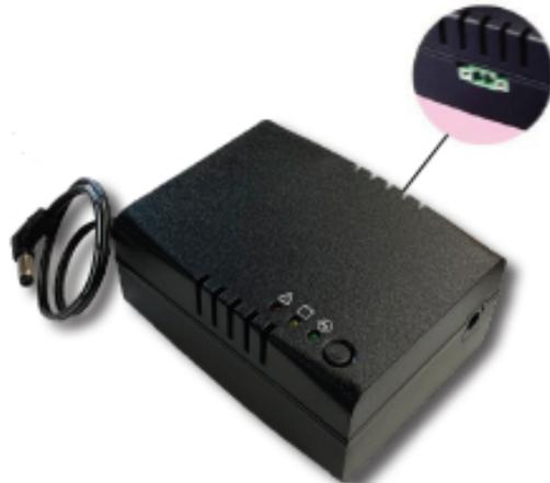
The POS36-10A can be used with a standard AC-DC desk top power supply to give battery back up in the event of an AC power failure. A 50W AC-DC power supply would be sufficient to charge the batteries and power the output at full load. So if you want 12V output you need a 12V input and so on. Powersolve have a range of suitable AC-DC adaptors for this purpose.
