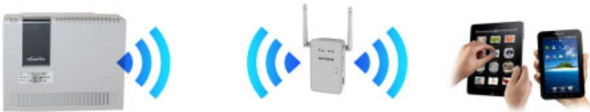
The primary drawback of a wireless repeater is that it effectively halves the bandwidth for any computers/devices connecting to it, rather than if they were connected direct to the router's WiFi. The reason for this is that the repeater receives the signal, processes the signal (which takes time) and then rebroadcasts the signal – and does this in both directions, from the router to the device and from the device to the router.
