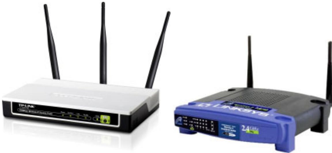
Above: examples of a wireless-N access points (AP). An AP can be connected by a long Ethernet cable to your B4RN router to provide strong broadband in areas of your house with poor WiFi signal..
