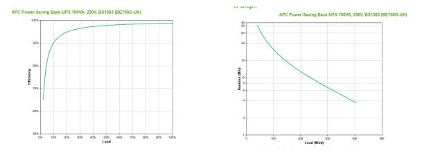
If only low power devices are connected to an AC UPS, like a router and Vonage adapter, the demand might only be 12Watts, at this level the efficiency might be as low as 65%.
