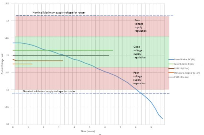
UPS Output Voltage Vs Time (22 Ohm load- nominal 6.5 Watt demand)
